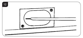
4.14 Remove the Compression Elbow from the appliance.
