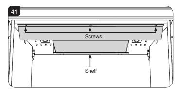
10.13 Replace the screws to secure it to the roof of the firebox, see Diagram 41.
