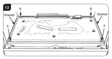
4.6 Remove the rear 2 corner screws, see Diagram 13, arrow B.
