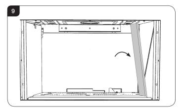
3.8 To remove the Left Hand liner first tilt inwards towards the centre of the firebox before lifting up and pulling out through the front of the firebox, see Diagram 9.
