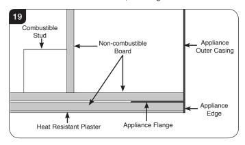
NOTE: If metal studwork is used, there is no need to fit non-combustible board to the face of the construction, see Diagram 20.
