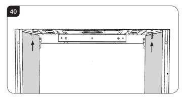
10.12 Replace the baffle ensuring that the rear locates on the shelf at the shelf at the back of the firebox, see Diagram 41. Take care not to damage the liners.
