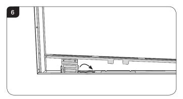
4.4 Remove the screws at the base of the glass frame, see Diagram 7 A.
