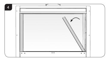
4.2 Lift out the bottom slotted trim, see Diagram 5.
