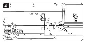
The injector can now be replaced.
