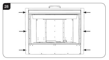
6a.6 Build the chimney breast up to coincide with the edge, allowing for the front to be skimmed level.
