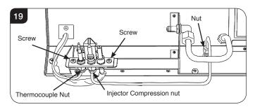
6.4 The pilot unit can now be removed and the pilot components can now be individually removed and replaced.
