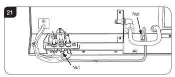
6.9 Remove the pipe and the injector drops out from the burner.
