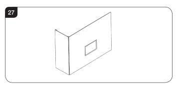
5.7 A removable access hatch must be left in the side of the chimney breast for future servicing and inspection of the appliance.
