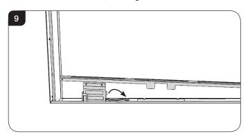
4.6 Remove the screws at the base of the glass frame, see Diagram 10 A.
