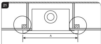
This diagram shows the minimum clearance position when installing the appliance into studwork - it is vital to ensure the batterning is wide enough to accommodate the fixings for the front.
