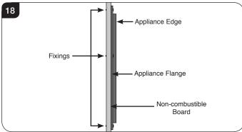
5a.10 Fit non-combustible board to the board around the appliance, see Diagram 13. Ensure distances to combustibles are observed, see Diagram 19.
